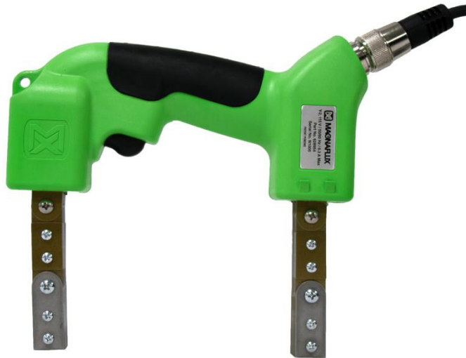
Slika 3-13. Električno napajana magnetska potkova ( https://irss.ca/ ,2022)
