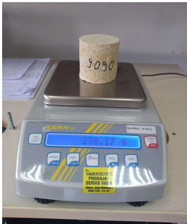
Figure 3-21. Test sample being weighted before drying
