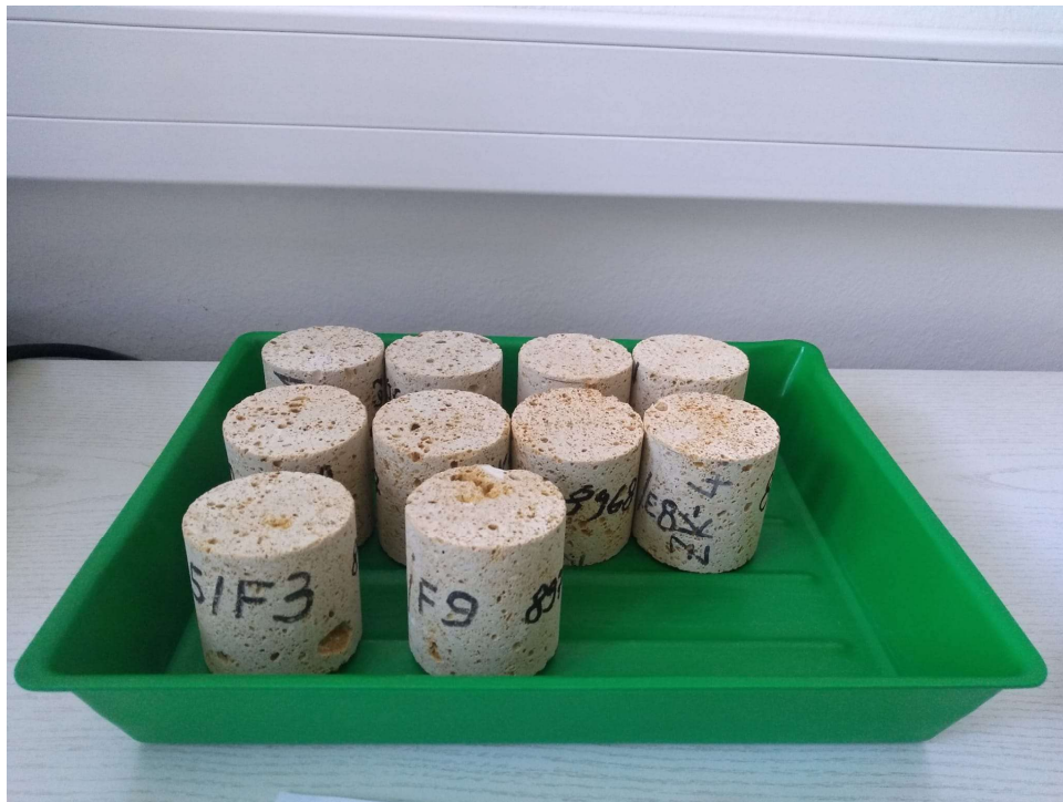
Figure 3-19. First set of samples before drying
