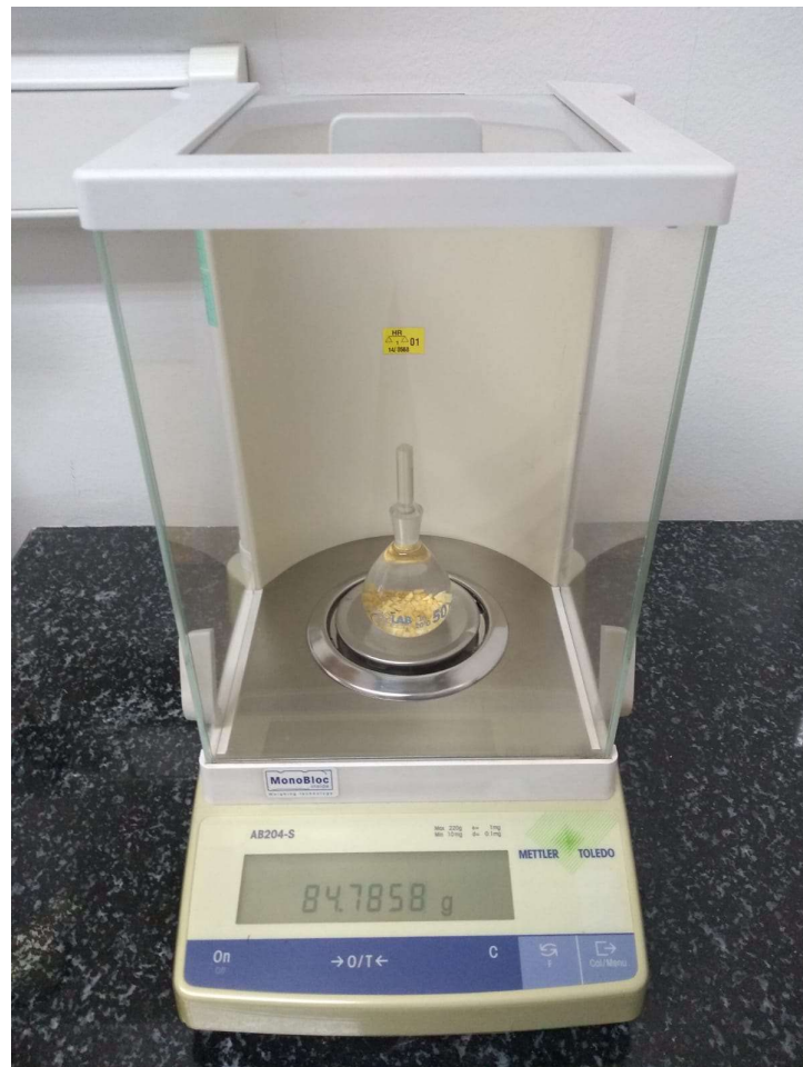
Figure 3-29. Now full pycnometer weighted
