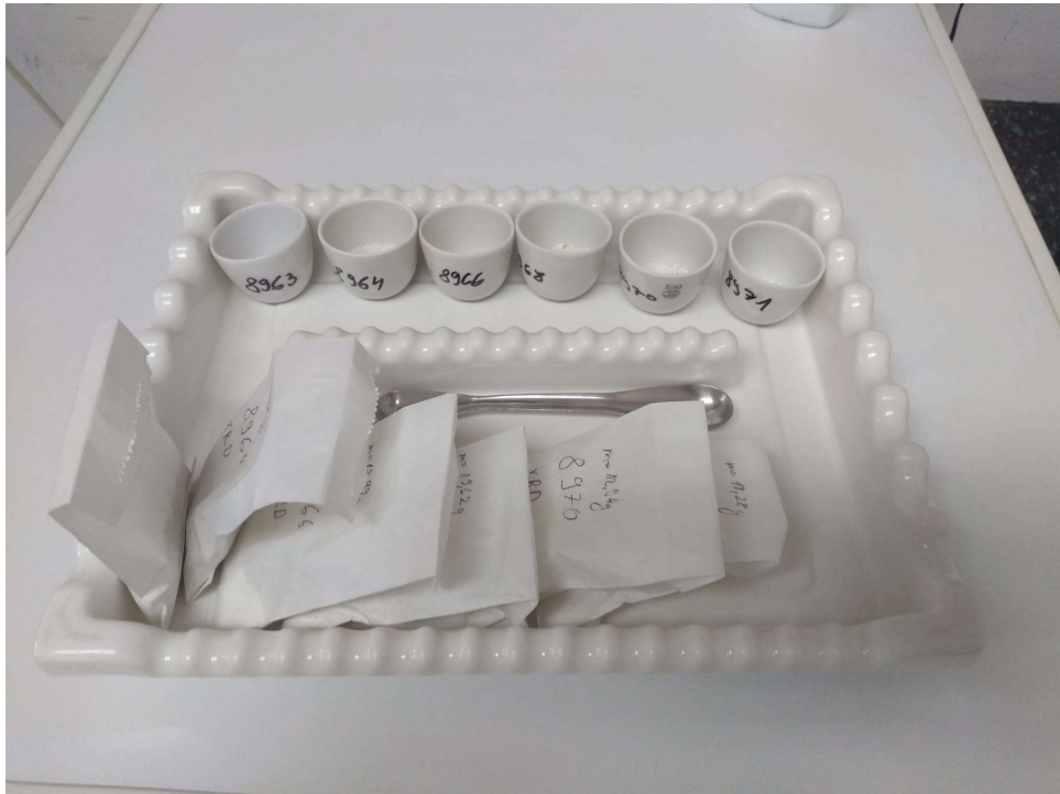
Figure 3-15. The powdered samples used for determining the moisture content
