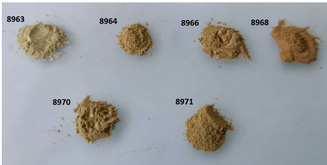
Figure 5-3. Insoluble residues after dissolving the carbonates in acetic acid
