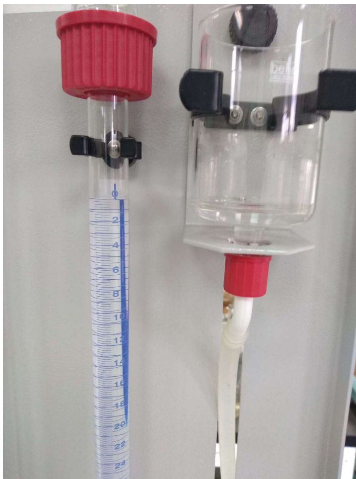
Figure 3-10. Calcimeter prepared for measurement: tube is filled to zero-mark before the hydrochloric acid reaction with sample and CO 2 release
