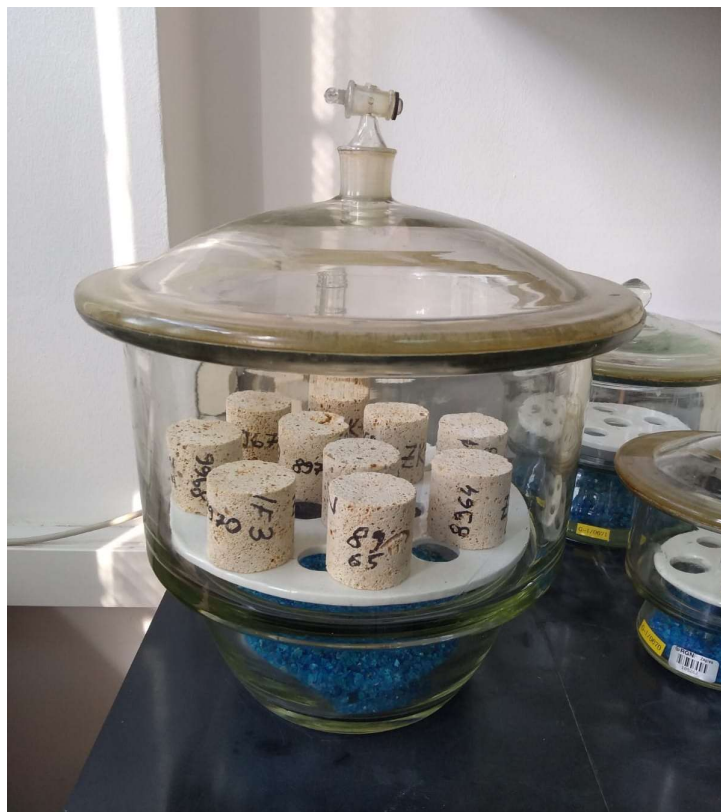
Figure 3-23. Test samples resting in a desiccator
