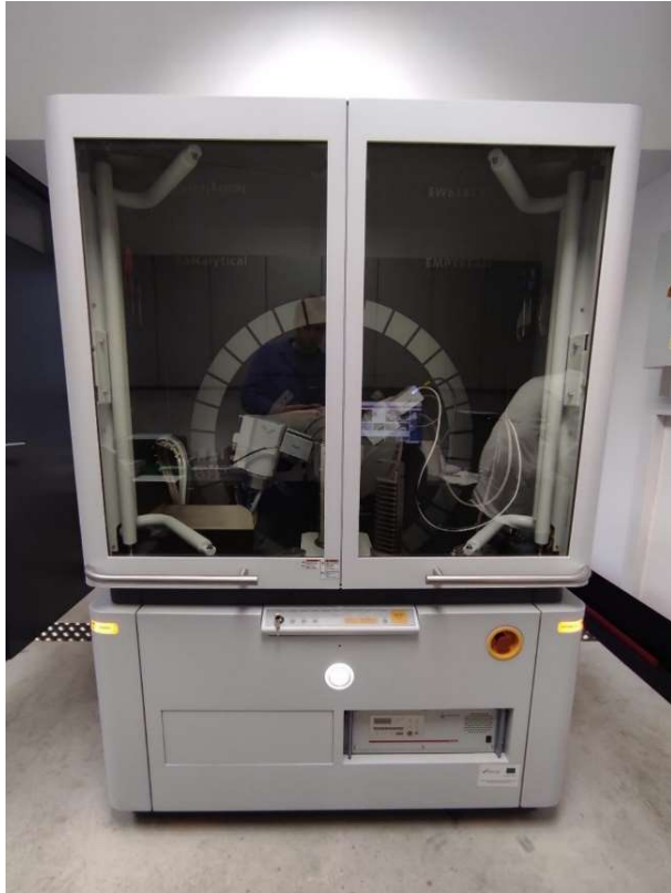
Figure 3-4. X-ray powder diffractor used in the study
