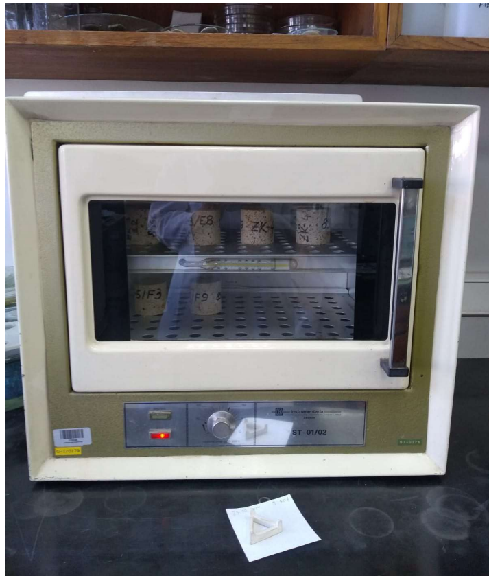
Figure 3-22. Test samples being dried
