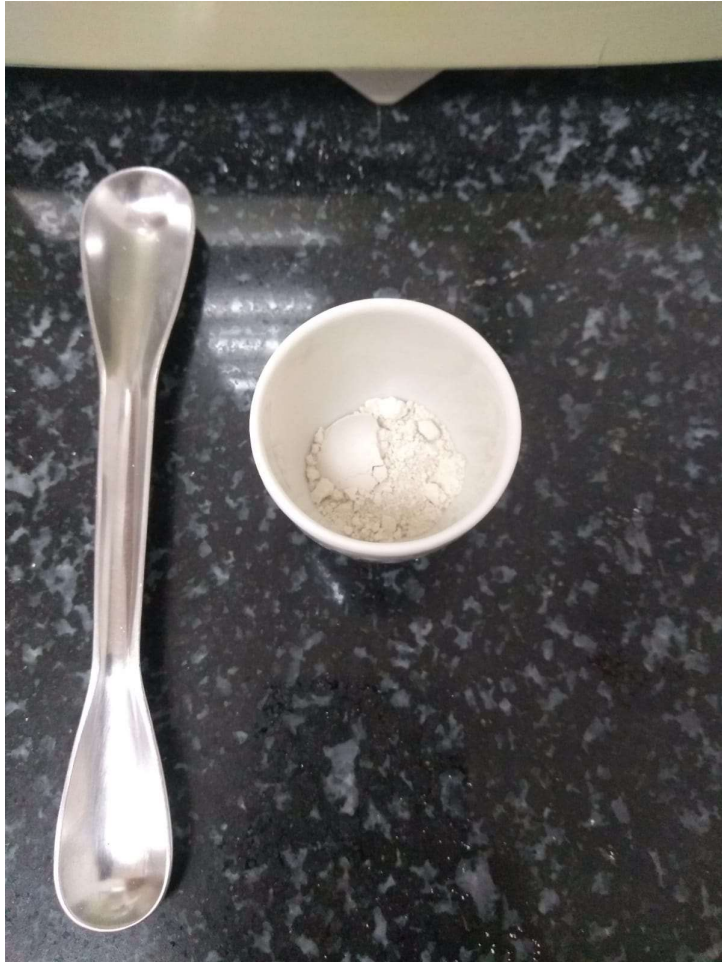
Figure 3-16. The powdered sample in crucible prior the heating
