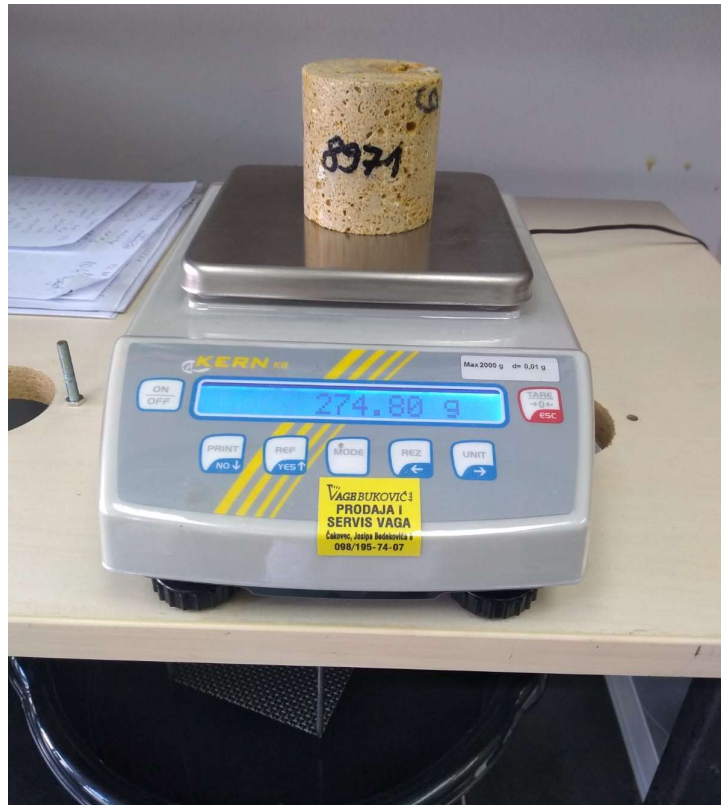
Figure 3-27. A fully saturated sample being weighted
