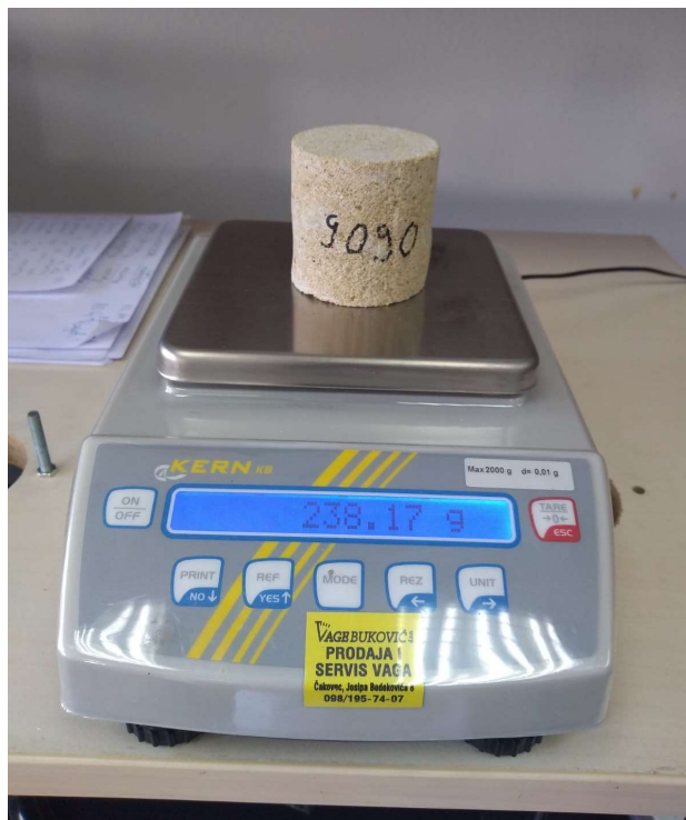
Figure 3-21. Test sample being weighted before drying
