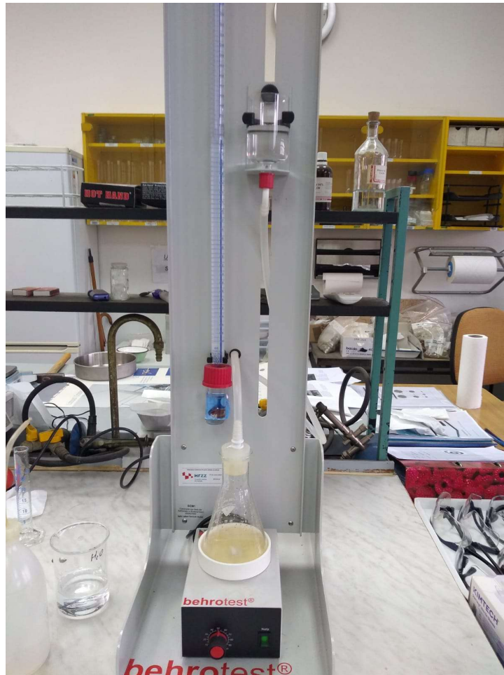
Figure 3-13. Apparatus after the CO 2 release
