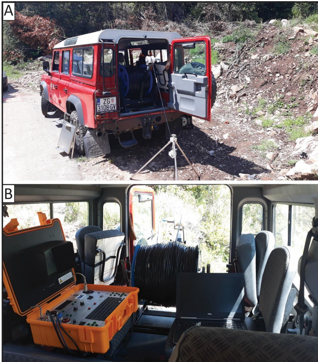
Figure 5. Borehole camera fieldwork configuration. (A) Terrain vehicle and tripod for centering of borehole camera; (B) operation console and winch for borehole camera.
