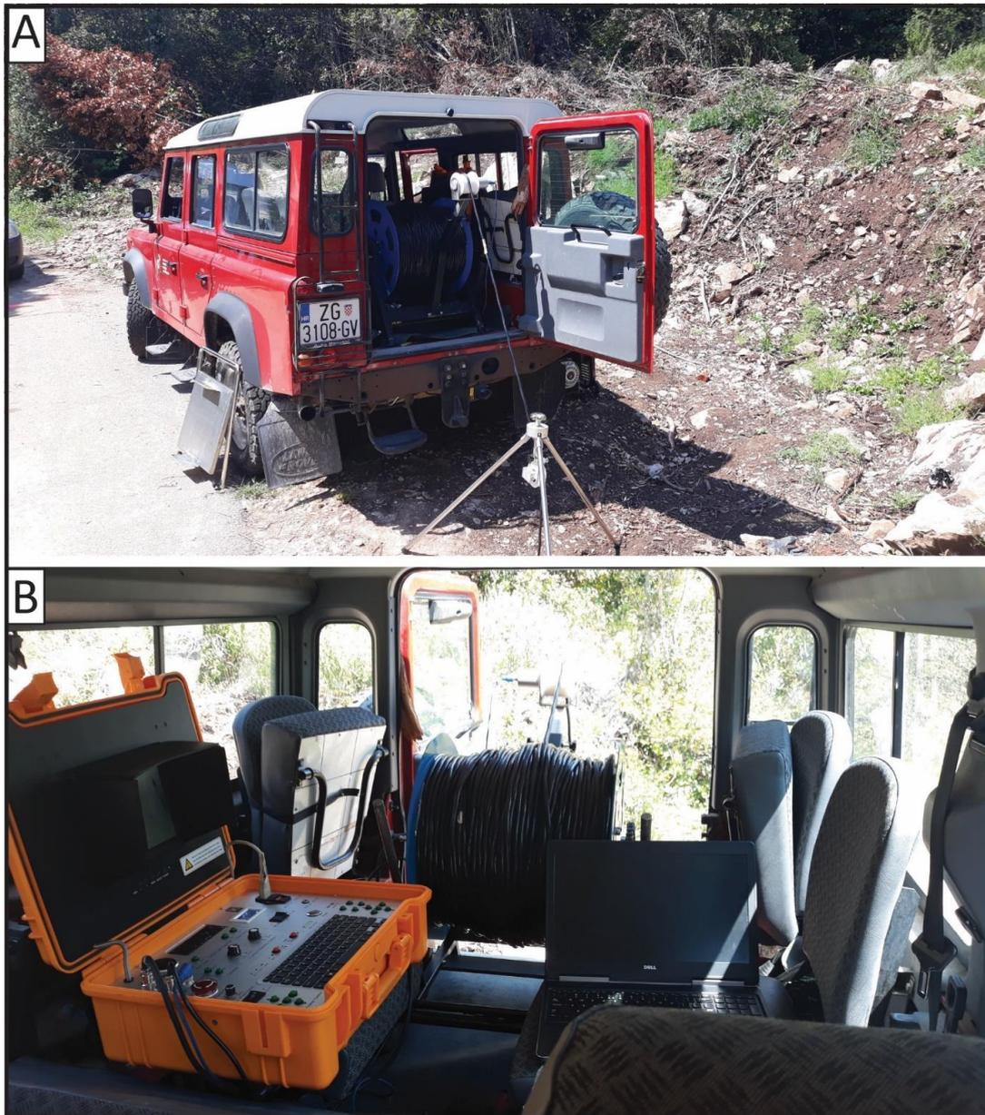
**Figure 5.** Borehole camera fieldwork configuration. (A) Terrain vehicle and tripod for centering of borehole camera; (B) operation console and winch for borehole camera.
