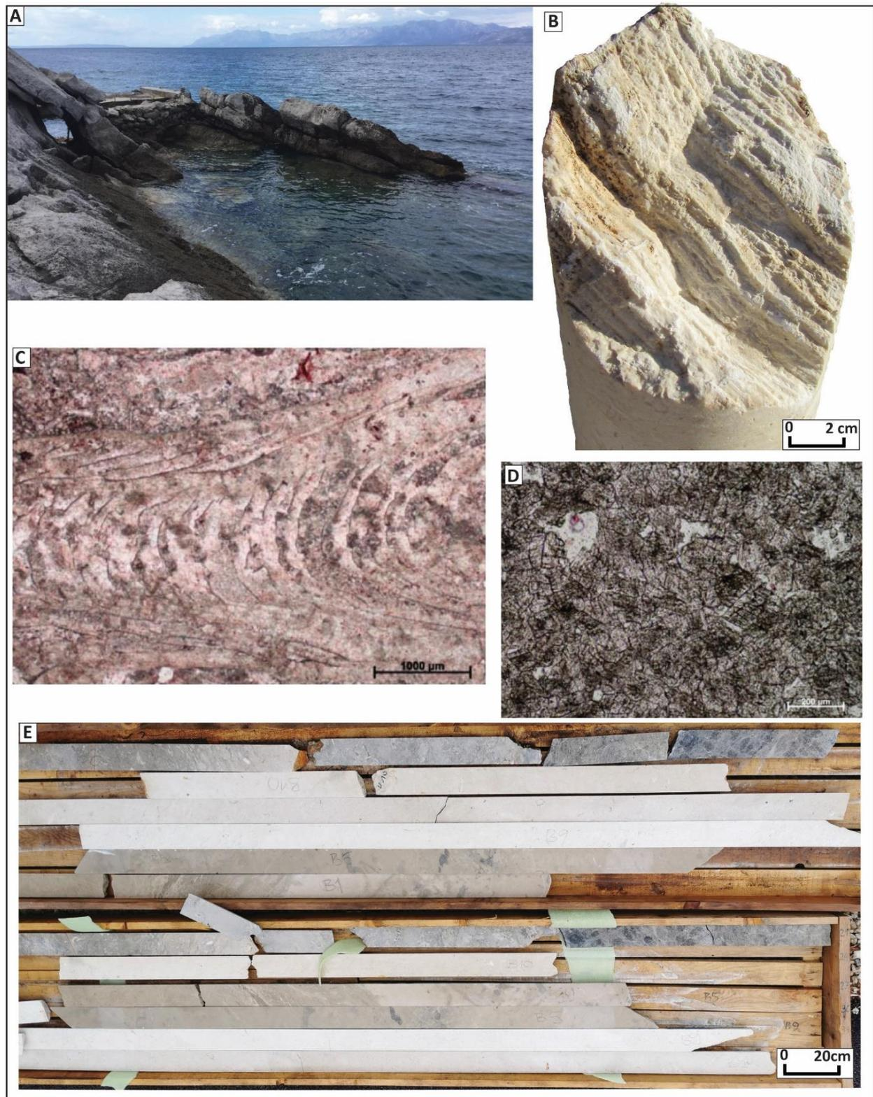
**Figure 2.** Shows (A) Upper Cretaceous limestones with 0.5–1 m thick layers in the northern part of Pelješac Peninsula; (B) Mollusk fossil in the drillcore; (C) microphotograph of fossiliferous limestone lithofacies; (D) microphotograph of late diagenetic dolomite lithofacies; (E) polished drill hole core samples of different lithofacies: white samples are micrite limestones, light gray to gray are fossiliferous limestones with bioturbations; dark samples are late diagenetic dolomites.
