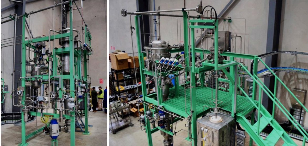
Figure 5-4. Hazer's pre-pilot plant in St Mary's, Sydney (Hazer Group, 2017a).
