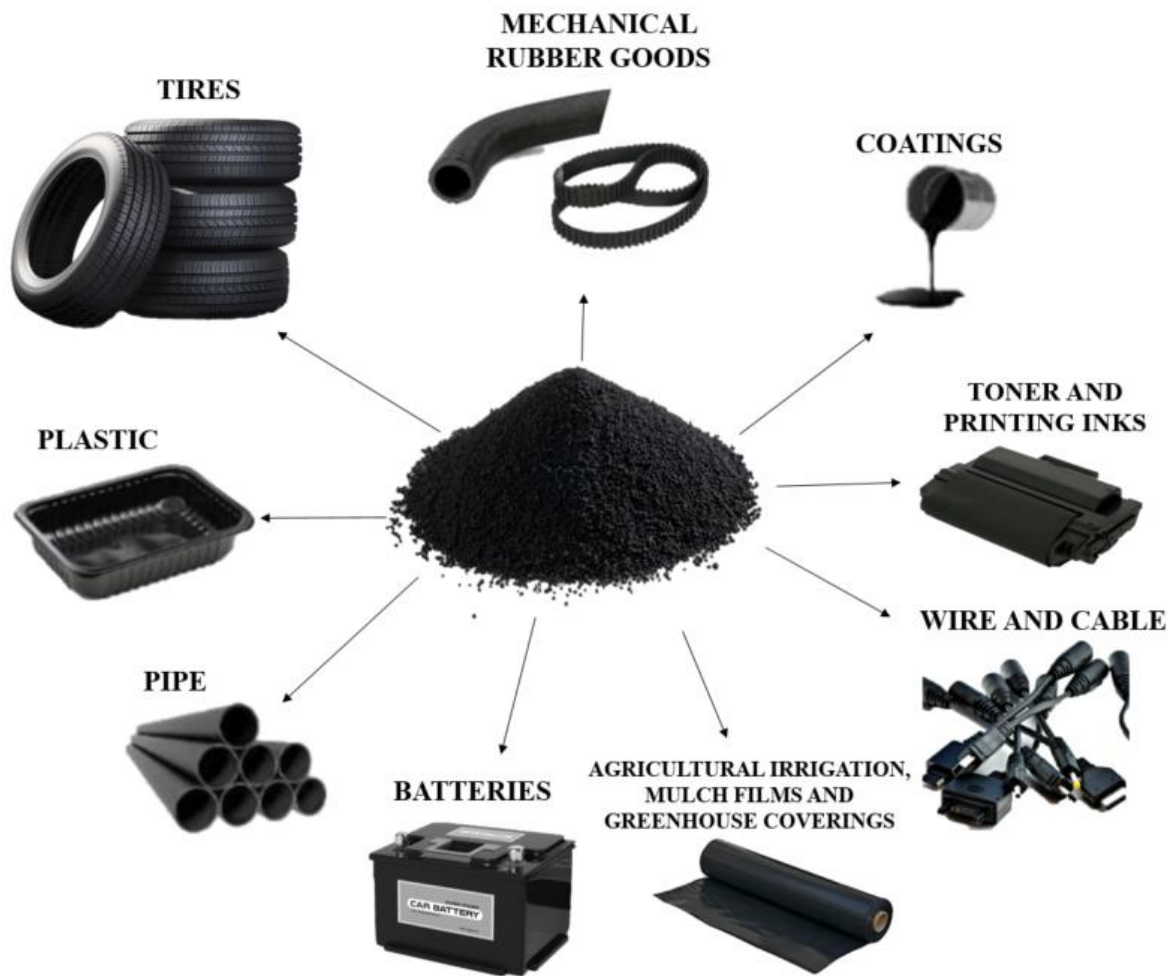
Figure 6-11. Examples of carbon black application (after Continental Carbon, 2014; ICBA, 2016; Orion Engineered Carbons, 2019c; Kouzegaran, 2020; ICBA, 2021; Mesrobian, 2022; Tek Toner, n.d.).
