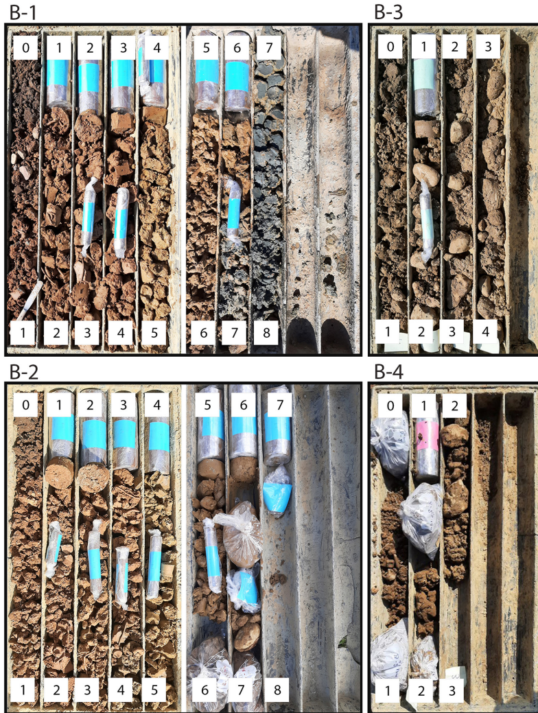
Figure 12. Soil core and sampling locations from boreholes B-1 to B-4 (photo by Evelina Oršulić). Numbers indicate depth in meters.
