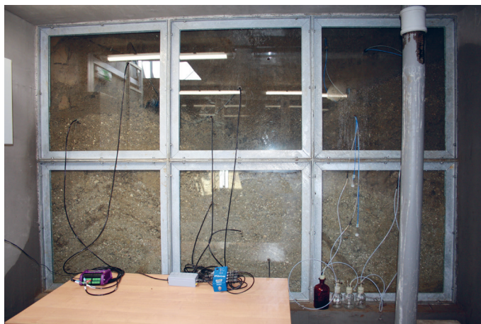
Figure 5. Eastern wall of the research pit with installed TDR probes (TP1 to TP6) – view from inside.
