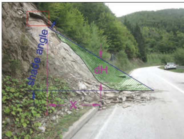
Figure 3 Cone model (red rectangle is source, black line is topographic surface, blue line is cone surface, shade angle ~ 32°, green area is a trajectory domain) of 2020 event in the background (photo M. Marjanović).
