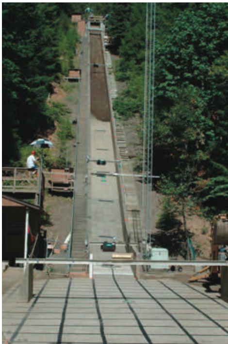
Figure 5 Photo of a 10 m 3 debris flow tested in the USGS flume (from Iverson et al., 2010).
