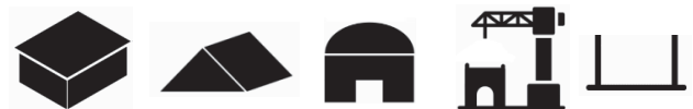
Most common typology of object roof type: flat; inclined; curved; unfinished/plate; without roof
