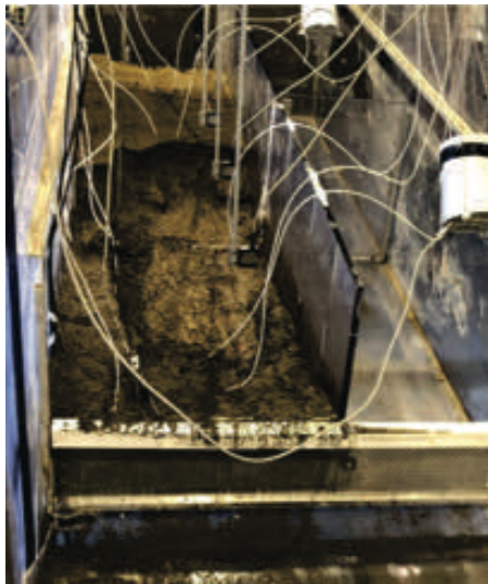
Figure 11 Detachment niche of the mudflow.
