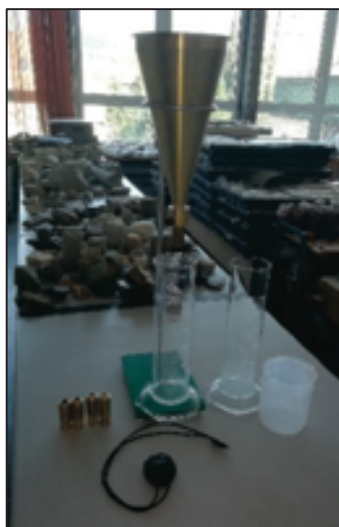
Figure 5 Funnel with different nozzle diameter.
