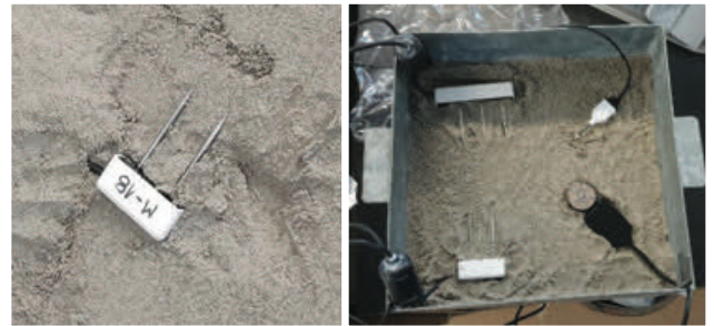
Figure 5 Installation of TEROS 10 during model build-up (left) and calibration for clean sand.
