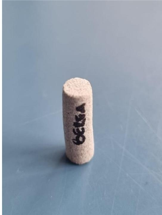
**Figure 3-3.** Drilled Berea sandstone sample.
