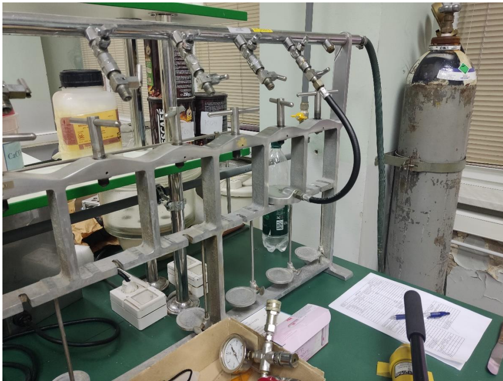
Figure 1-1. API filter press
