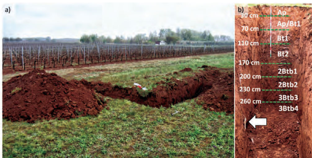
Fig. 22. (a) Terra rossa soil profile located in a vineyard at Koreniki (northwest coast of the Istrian peninsula, Croatia). (b) Cleaned terra rossa soil profile overlying a lower Eocene foraminifera limestone (marked by white arrow) with Ap, Ap/Bt1, Bt1, Bt2, 2Btb1, 2Btb2, 3Btb3 and 3Btb4 horizons.
