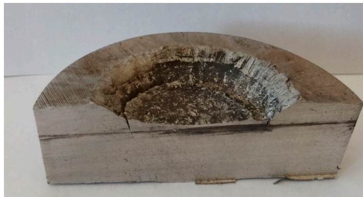
Figure 3. Aluminum plate cross-section after testing.
