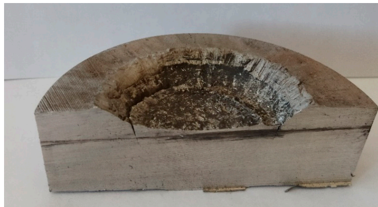
Figure 3. Aluminum plate cross-section after testing.
