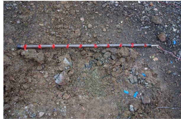
Fig. 3. The steel-charge detonation velocity measurement setup.
