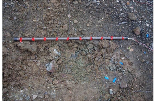
Fig. 3. The steel-charge detonation velocity measurement setup.
