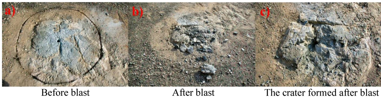
Fig. 8. The crater formed with the largest specific breakage (M + EPS 40:60).
