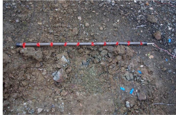
Fig. 3. The steel-charge detonation velocity measurement setup.
