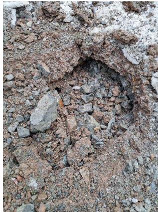
Figure 4. Blast performance for bore hole charged with 40:60 mixture
