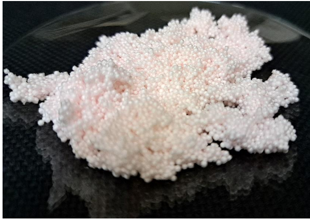
Figure 3. Low-density emulsion matrix based mixture
