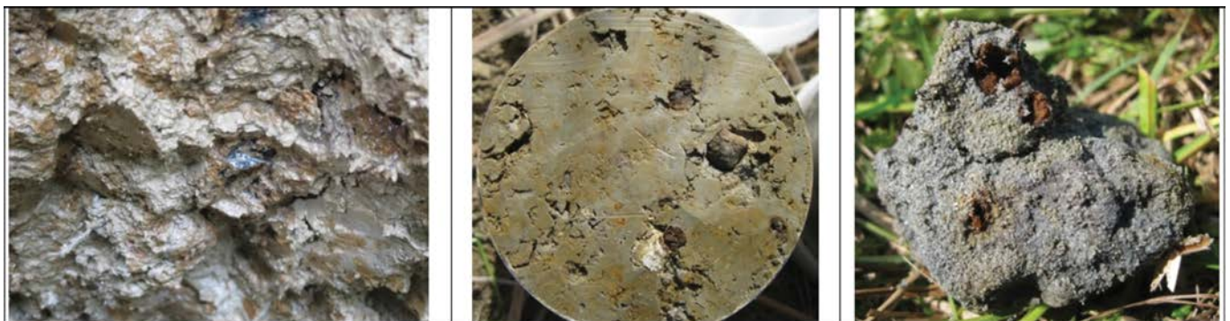
Figure 2. (Source: Vedran Rubinić). Left: A detail (in reality, photograph is 12 cm wide) of the in situ morphology of a soil horizon with stagnic properties. Masses and linings (coatings) of reprecipitated iron (brown to orange) and manganese (black) represent soft redox concentrations. Albic material (grey) represents reduced matrix parts (sporadically) or local depletions of iron (mainly). Middle: Cross section of a core sample (in reality, photograph is 5 cm wide) taken from a soil with both stagnic and gleyic properties. One can observe fine, light brown to orange, soft masses along the larger, darker, and more cemented nodules/concretions of iron and/or manganese. Redox concentrations are mostly surrounded by greenish-gray soil matrix, which is reduced and/or iron-depleted. The white spot on the surface of the sample is a cut off concretion of calcium carbonate. Right: A clod from a soil profile with gleyic properties. Soil matrix is reduced (almost entirely bluish gray, probably due to the presence of vivianite), whereas along the root channels iron reprecipitates to form oxidized rhizospheres (light orange colors).
