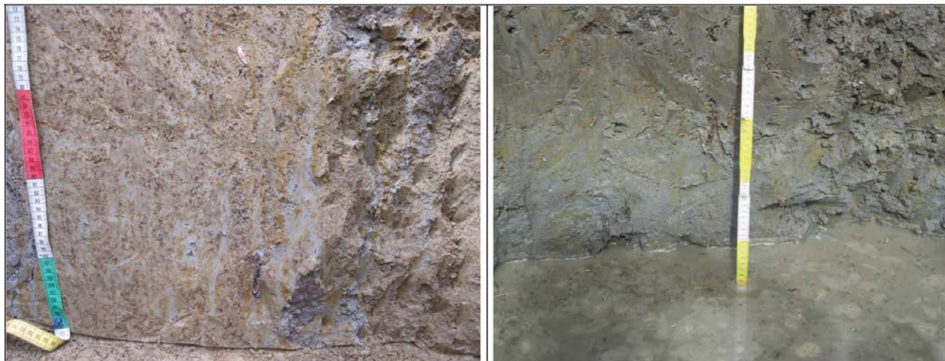
Figure 6 (Source: Vedran Rubinić). Left: Mottled morphology of a soil horizon with stagnic properties (pseudogleization). Oximorphic colors (mostly black, orange, and dark brown mottles) predominate over reductimorphic colors (albic material), which occur mainly as vertical tongues (albeluvic glossae). Right: Reductimorphic colors, formed due to high groundwater in the soil profile, point to gleyic properties.
