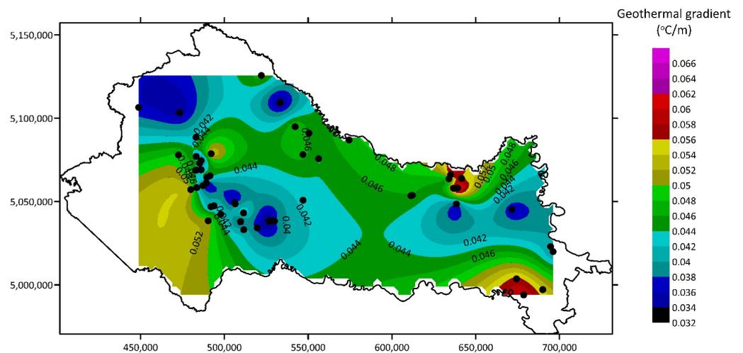
Figure 13. Geothermal gradient map for post-rift phase.
