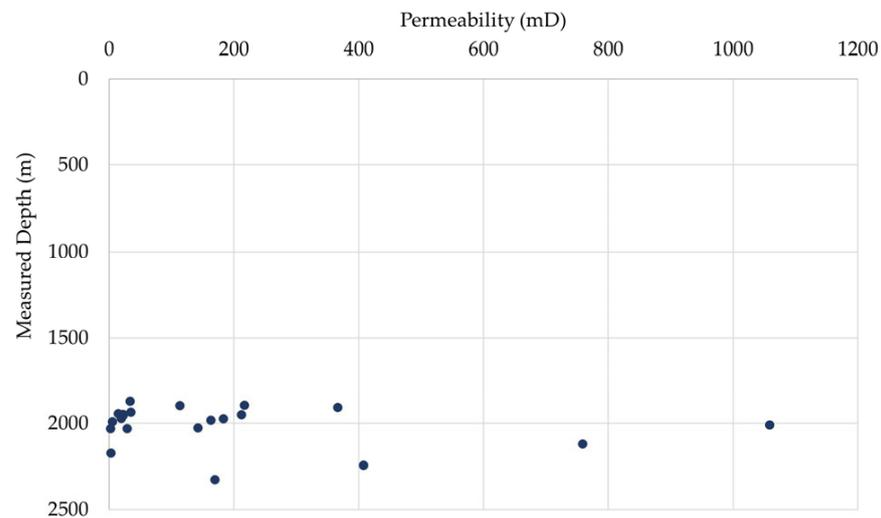
Figure 7. Permeability of wells determined using DST measurements.
