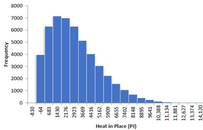
Figure 11. Heat-in-place probability distribution for well doublets—syn-rift phase.
