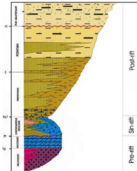
Figure 1. Schematic geological column of the Pannonian basin (Durn & Krpan, 2016; Saftić, et al., 2003)
