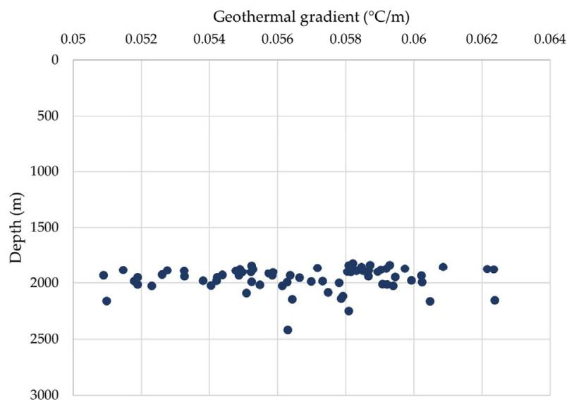
**Figure 5.** Geothermal gradients across the oil field wells.
