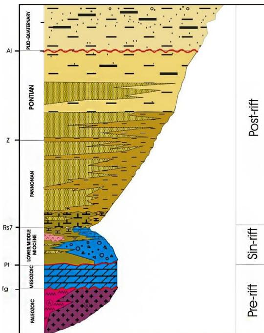
**Figure 2.** Schematic geological column of the Pannonian basin [53,61].
