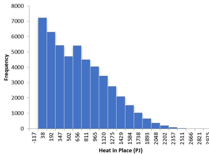
**Figure 10.** Heat-in-place probability distribution for well doublets—post-rift phase.
