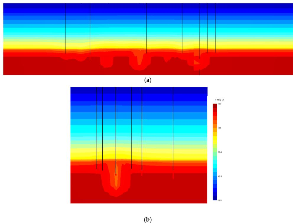
**Figure 15.** Cold front distribution in Scenario 2 after 30 years of production ((a) front view; (b) side view).
