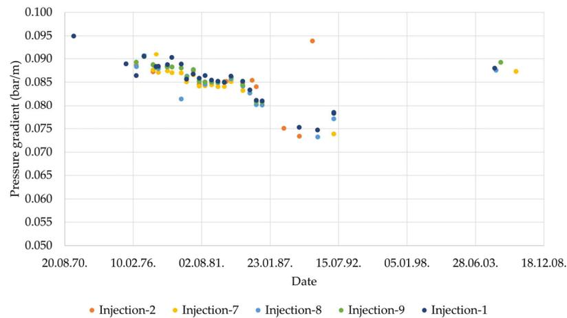
**Figure 4.** Pressure gradient measurements of injection wells during oil production.
