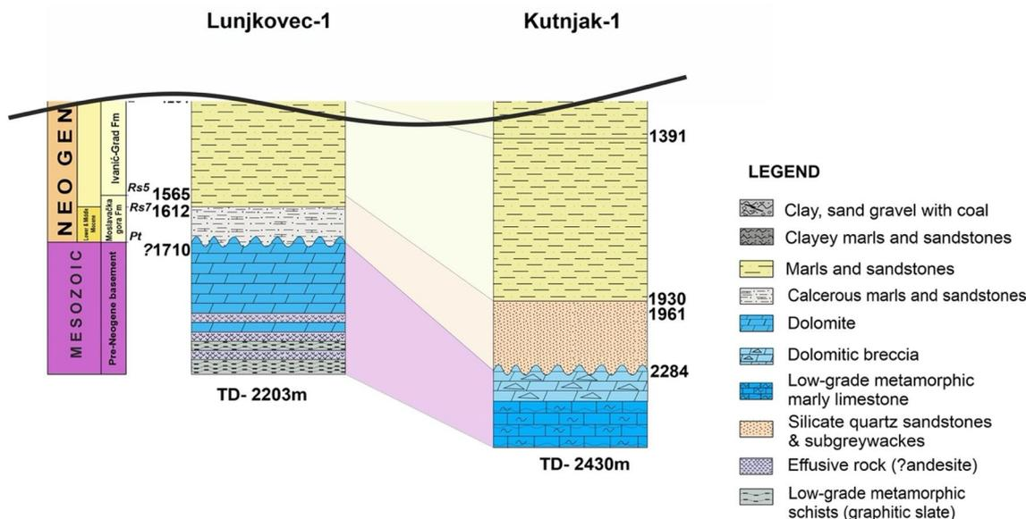
Fig. 18 Schematic lithostratigraphic column of wells Lunjkovec-1 and Kutnjak-1 (Croatian Hydrocarbon Agency 2020a, b, c, d, e)
