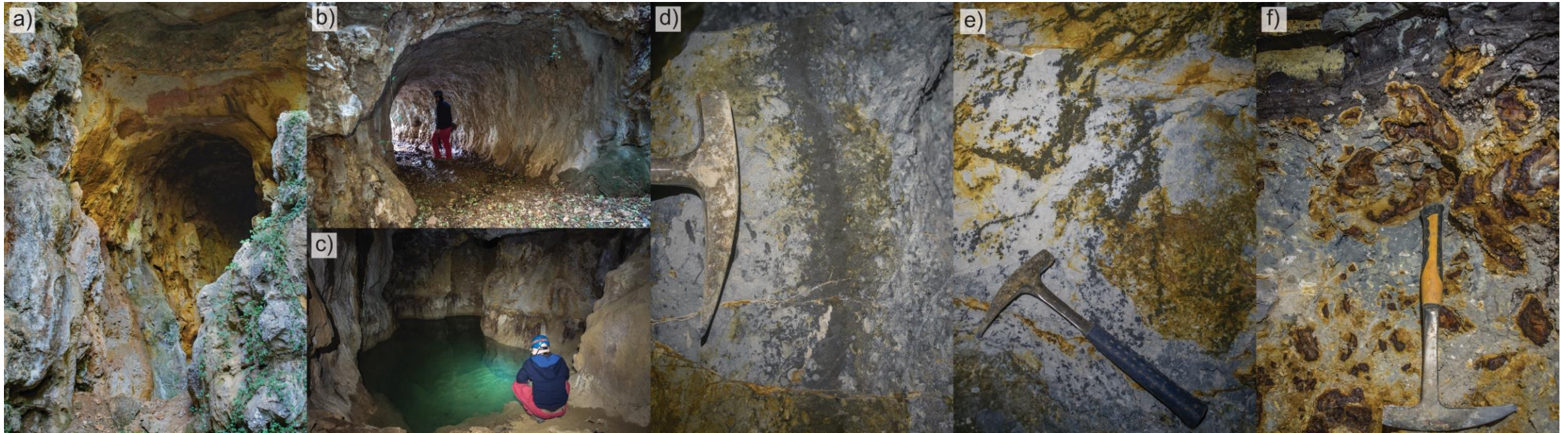
Figure 6. Field photographs of Minjera bauxites a) D-5 bauxite deposit, b) Entrance shaft into the D-7 bauxite pit, c) Lake in the D-3 bauxite deposit, d) Transition from the grey bauxite into the black bauxite and Kozina beds, e) Iron sulphide veins, f) Iron sulphide impregnation
