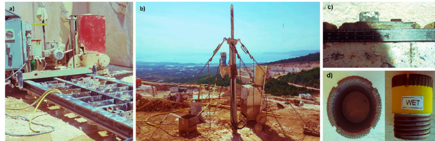
Figure 1. (a) Chain saw; (b) Hydraulic rotary drill; (c) Cutting tool; (d) Natural diamond core bit.
