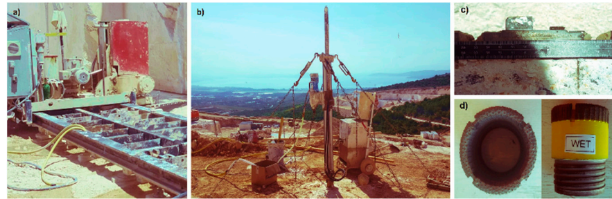
Figure 1. (a) Chain saw; (b) Hydraulic rotary drill; (c) Cutting tool; (d) Natural diamond core bit.
