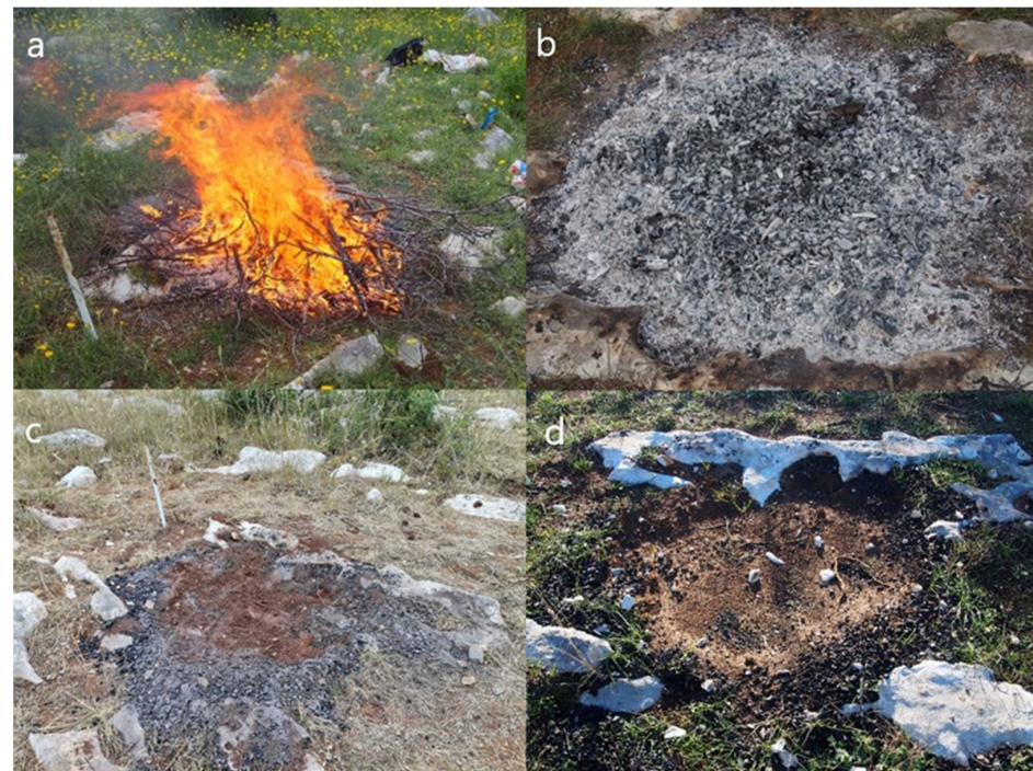
Figure 2. (a) Burn experiment, (b) immediately after the fire, (c) one month after the fire, (d) six months after fire.
