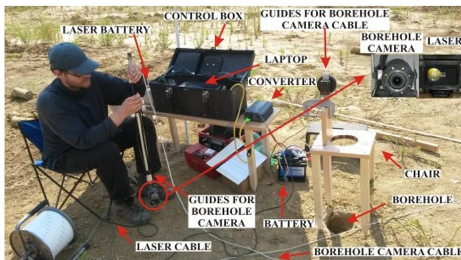
**Figure 2.** Developed integrated borehole camera laser system [4].
