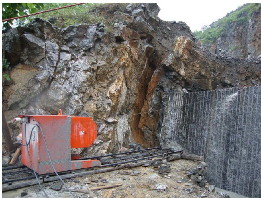
Slika 2-21. Dijamantna žična pila pri radu ( https://www.xmsinostar.com/wp-content/uploads/p2-diamond-wire-saw-machine-for-marble-quarry-cutting.jpg )
