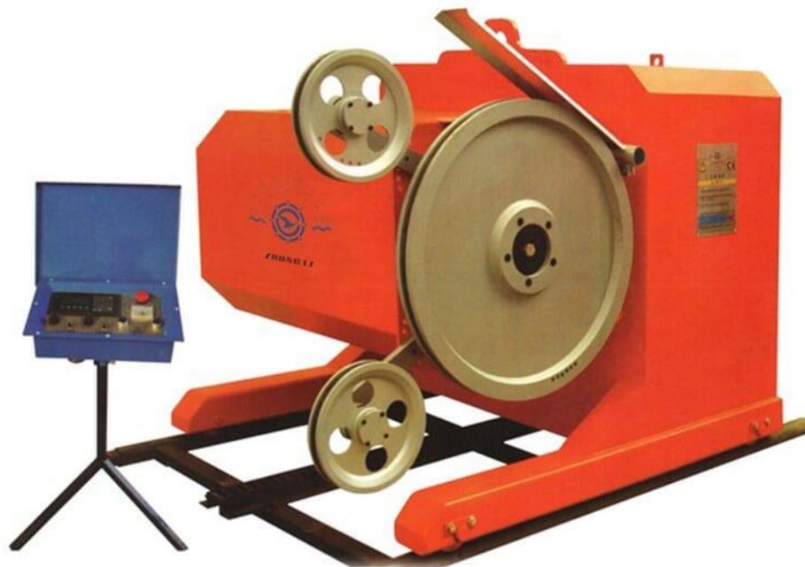
Slika 2-19. Postrojenje dijamentne žične pile ( https://www.xmsinostar.com/wp-content/uploads/Diamond-Wire-saw-machine-for-marble-granite-quarry.jpg )
