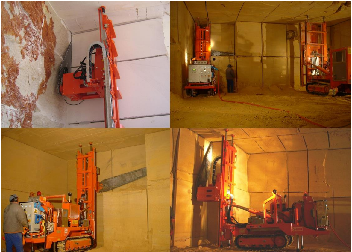
Slika 2-4. Lančana sjekačica Fantini Model SV50 ( https://www.fantinispa.it/en/svc50-tunnel-chain-saw-machine/ )
