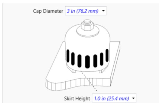
Figure 2-5 Illustration of a bubble cap on a tray from the column internals menu in HYSYS
