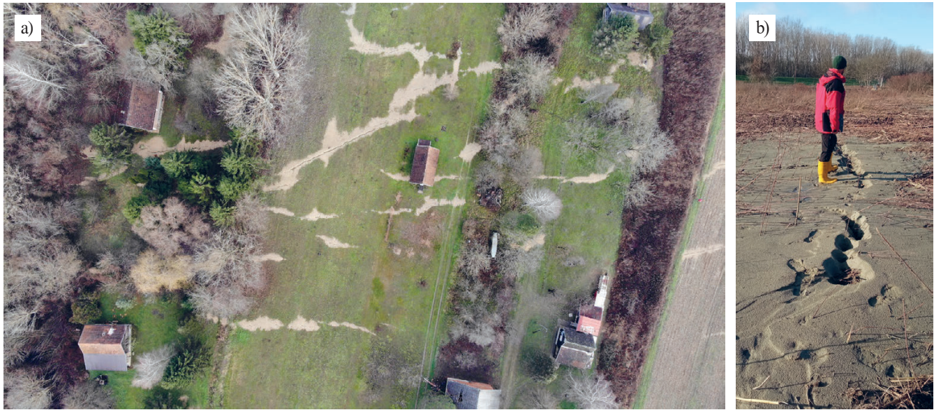
Figure 5. The sand boiling features along linear fractures: a) in Letovanić (aerial photo); b) in Sisak (observation point Si-04).
