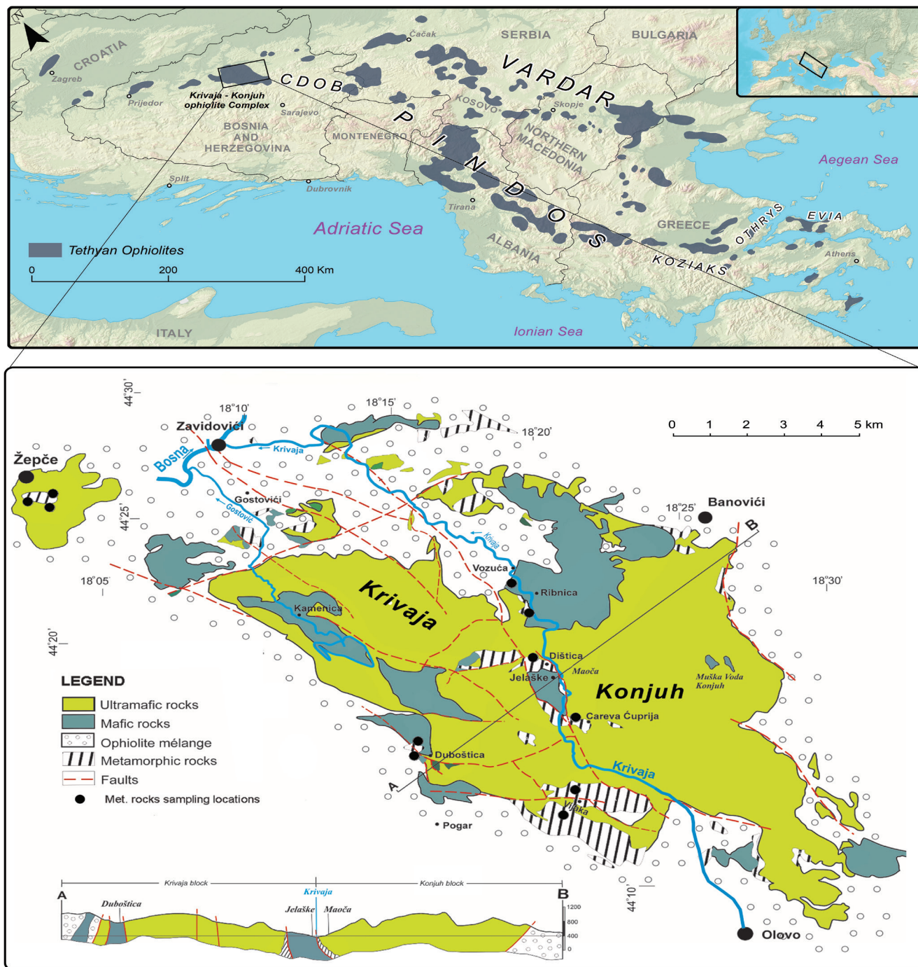
Figure 1. Upper part: A geotectonic schematic map of SE Europe showing the Mesozoic Tethyan ophiolites stretching parallel to the Dinarides. The rectangle indicates the position of the Krivaja-Konjuh ophiolite complex (study area). Map modified after ROBERTSON (2002) and ŠEGVIĆ et al. (2019); Lower part: A simplified geological map of the Krivaja-Konjuh ophiolite complex. Modified after PAMIĆ (1968; 1970), ĐORĐEVIĆ and PAMIĆ (1972), and ŠEGVIĆ et al. (2019). The SW-NE cross-section A-B depicts the tectonic nature of the contact between large blocks of ultramafites and subordinate mafic rocks.
