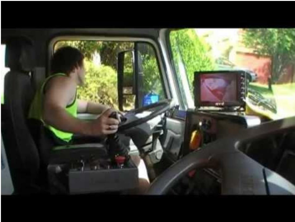
Figure 9-5. An example of the inside of the cabin of a Raptor Side Lift truck (MitchellM15, 2013).
