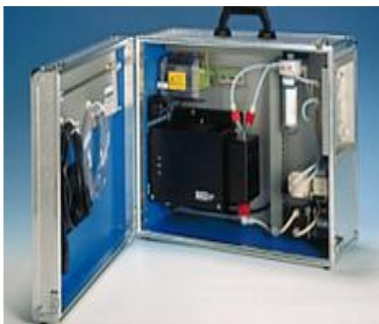
Slika 4-21. Peltier hladnjak (EKONERG d.o.o., 2015)
