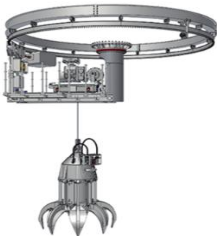
Slika 6-5. Dh DG 500 (Deilmann-Haniel Mining Systems, 2016)
