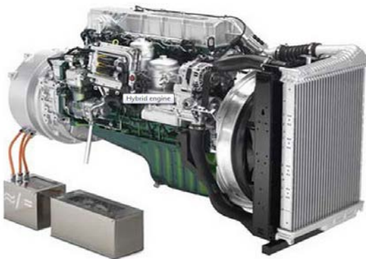
6-13. Prikaz motora hibridnog kamiona ( http://www.volvotrucks.com )
