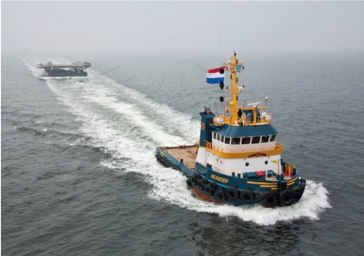
Slika 2-14. Oceanski remorker ( engl. offshore towboat ) ( www.landfall.nl )
