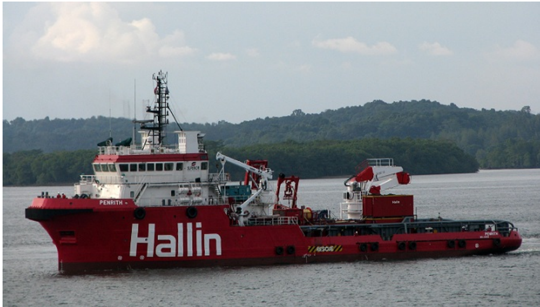
Slika 2-1. Plovilo za potporu uronima ( www.maritime-connector.com )
