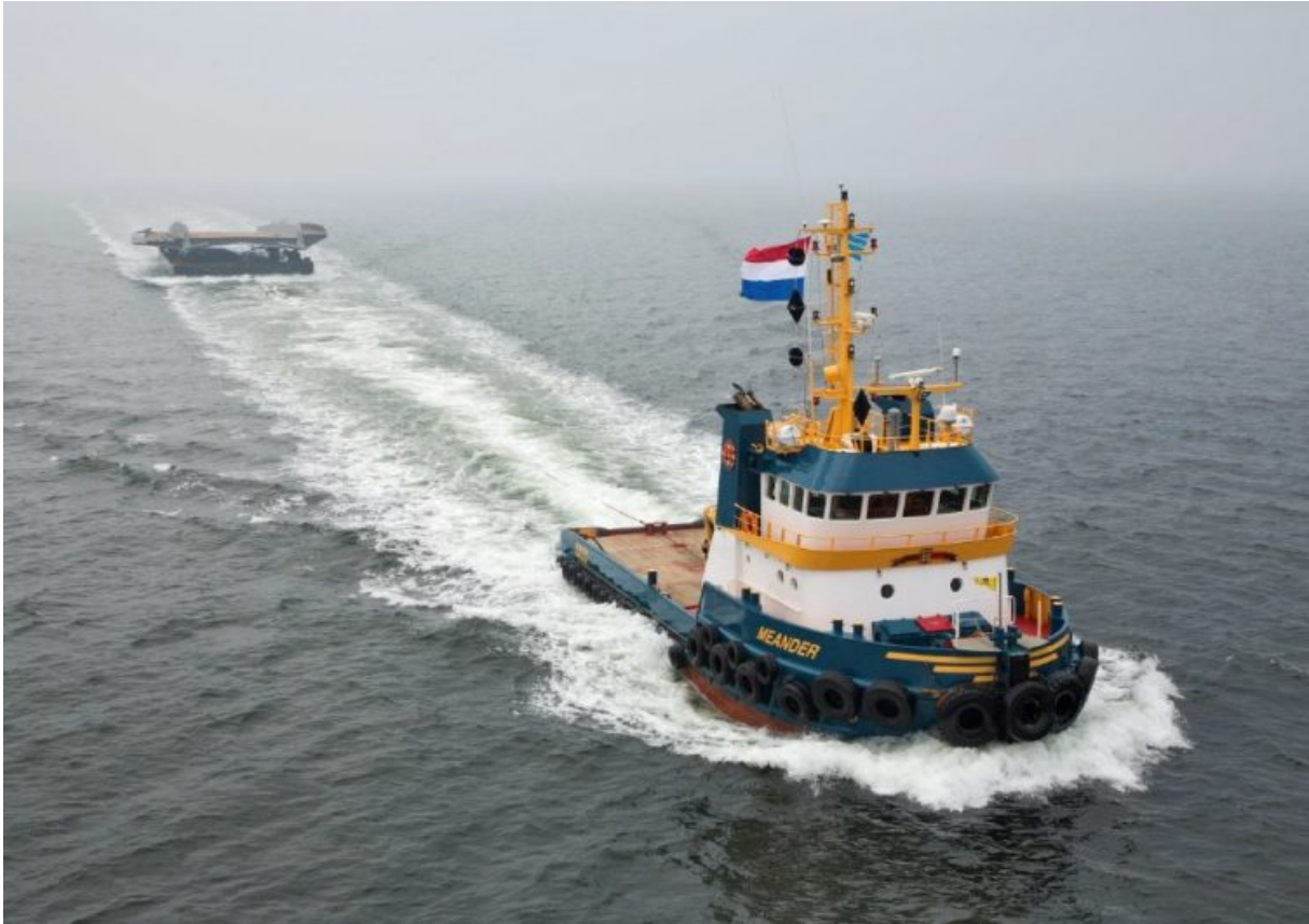
Slika 2-14. Oceanski remorker ( engl. offshore towboat ) ( www.landfall.nl )
