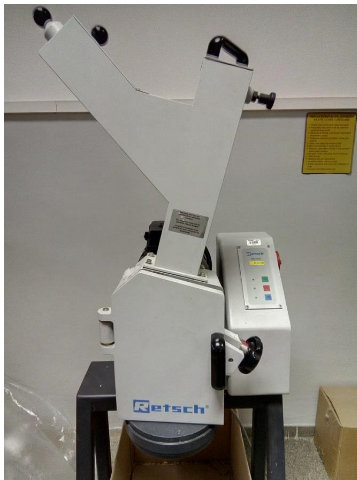
Slika 6-4 Rezni mlin (Cutting Mill RETSCH SM 2000)
