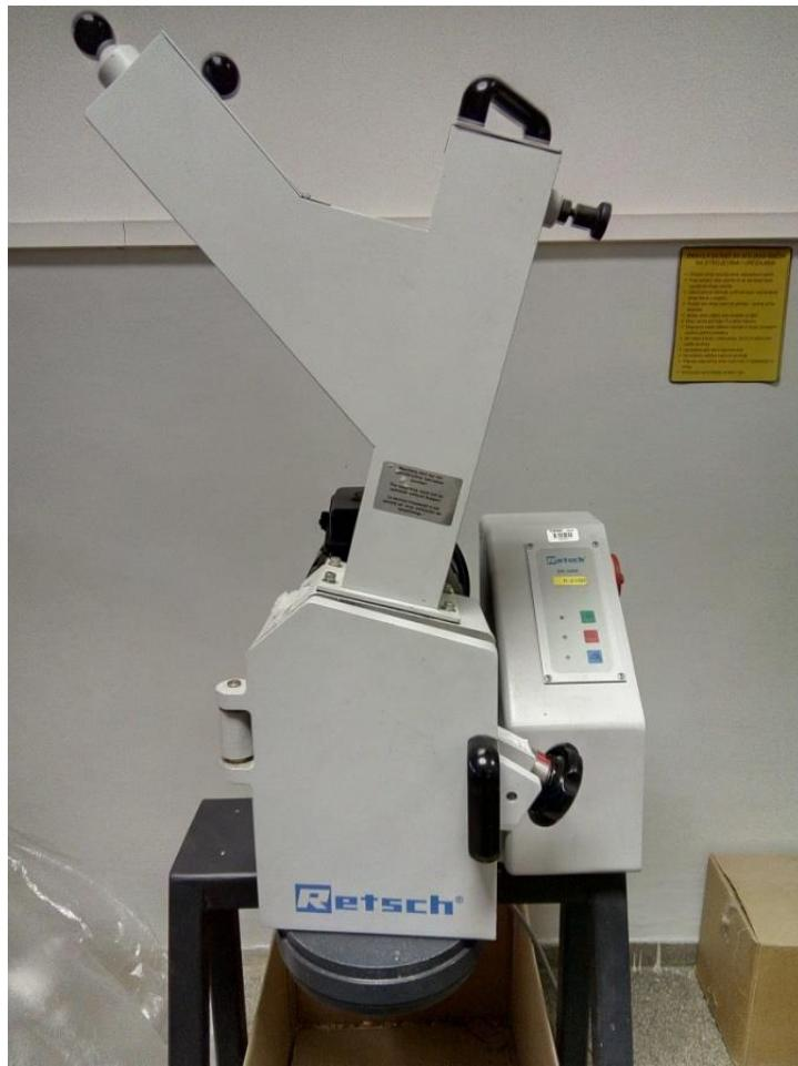
Slika 6-4 Rezni mlin (Cutting Mill RETSCH SM 2000)
