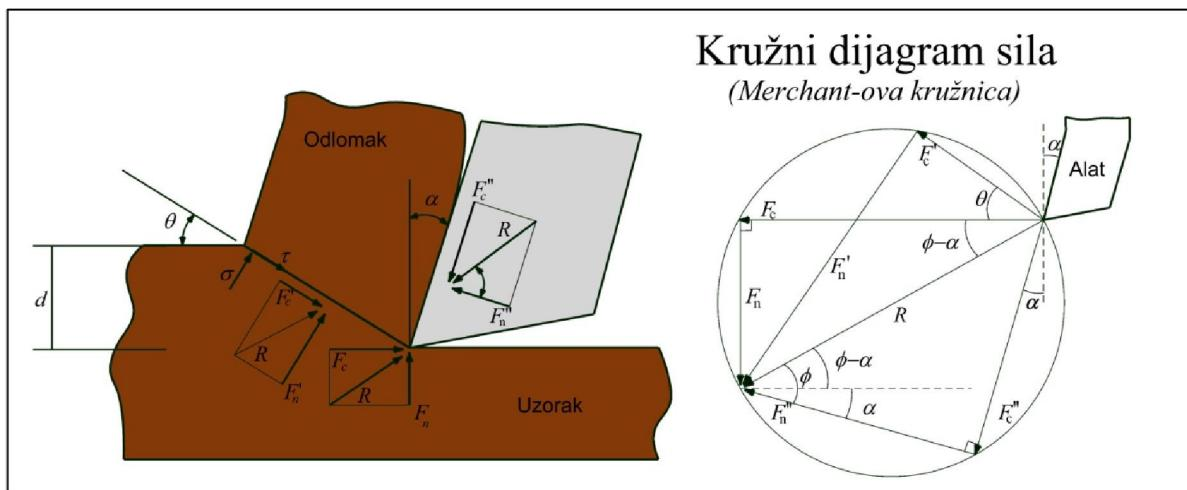
Slika 3.3. Merchant-ov model i kružni dijagram sila (Merchant, 1945).
