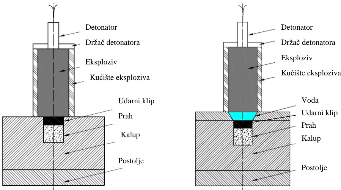
Slika 3-12. Kompaktiranje prahova metodom udarnoga klipa (Zohoor & Mehdipoor 2009)
