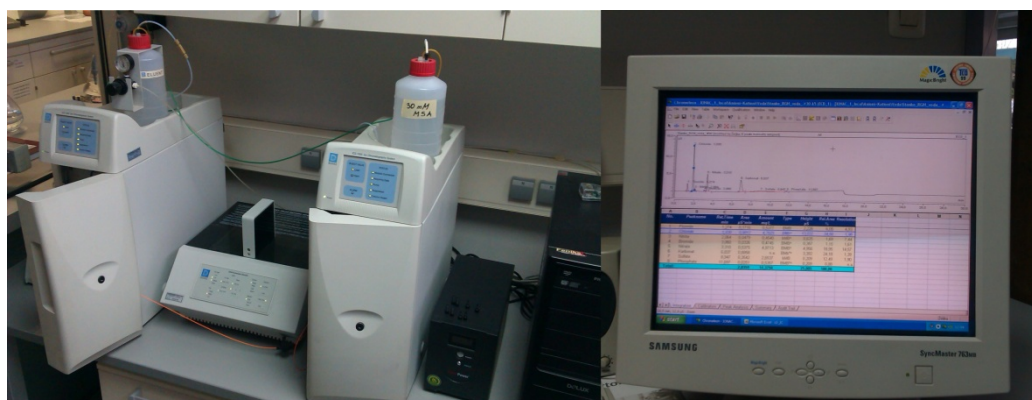
Slika 5.22. Dionex ICS–1000 Ion Chromatography System i anionski kromatogram (Chromeleon®software, Version 6.60 Build 1428, Dionex Corporation).
