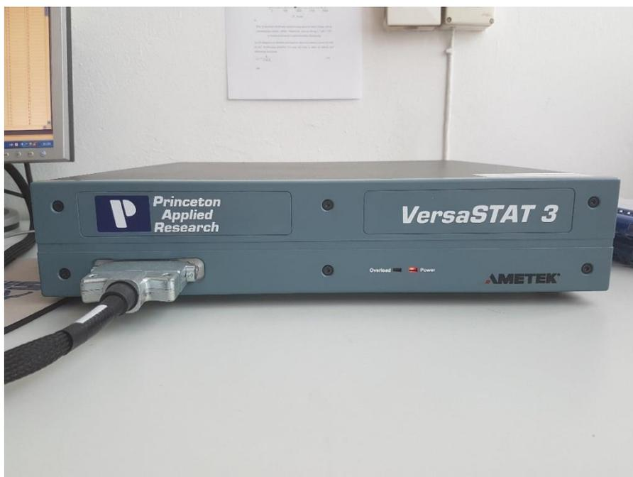
**Slika 5-13.** Potenciostat (Princeton Applied Research model VersaStat 3)
