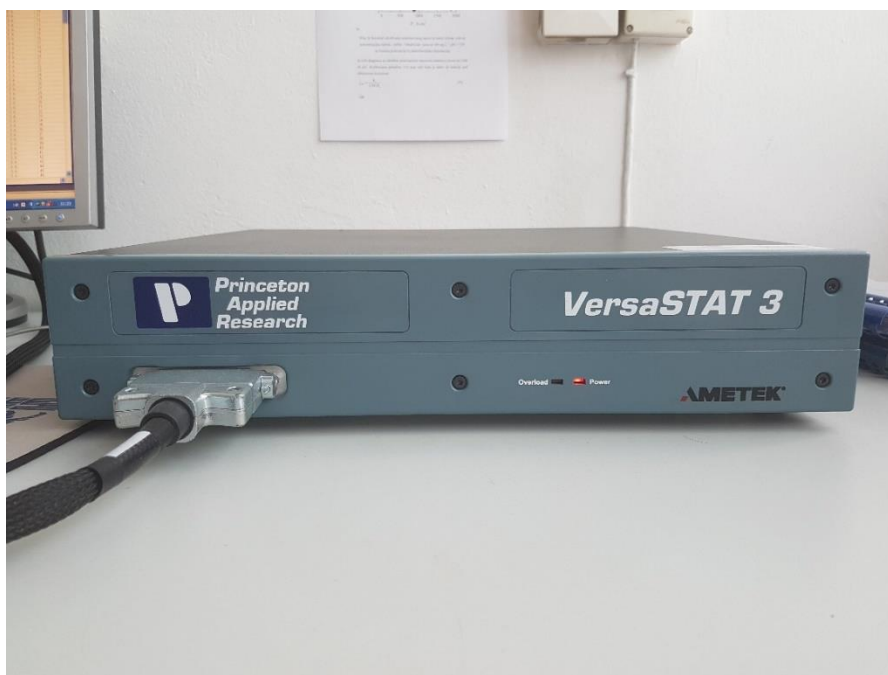
Slika 5-13. Potenciostat (Princeton Applied Research model VersaStat 3)
