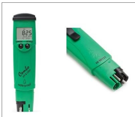
Slika 5.1. HI98121 pH/ORP/Temperature Combo Tester (Hanna Instruments, 2017).
