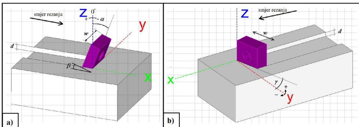
**Slika 2-7** Geometrijske veličine reznog alata a)  $\alpha = -20^\circ$ ,  $\gamma = 0^\circ$ ,  $\delta = 0^\circ$ ,  $\beta = 20^\circ$ ; b)  $\alpha = 0^\circ$ ,  $\gamma = 15^\circ$ ,  $\delta = 0^\circ$ ,  $\beta = 0^\circ$  (Korman, 2014).
