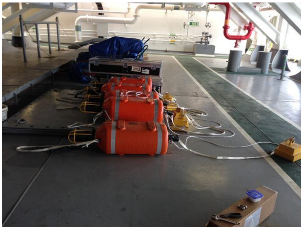
Slika 3-7. Transponderi (Pacific Drilling, 2009)
