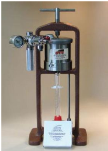
Slika 5-10. API filter preša (OFI Testing Equipment, 2018 (e))
