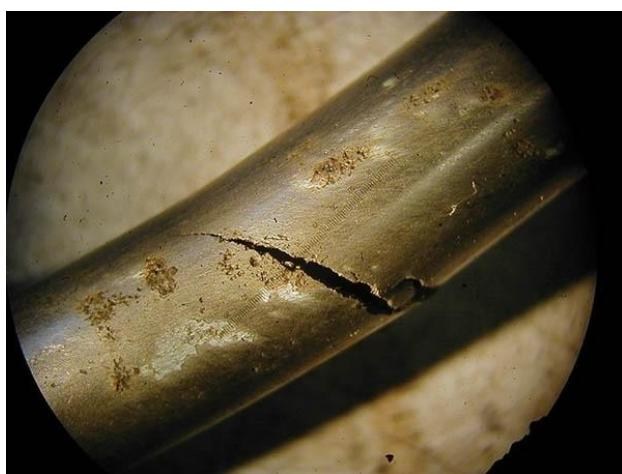
Slika 2-2. Primjer pukotinske korozije (Sachs, N. 2018, Efficient Plant, Corrosion: Understand It to Fight It)
