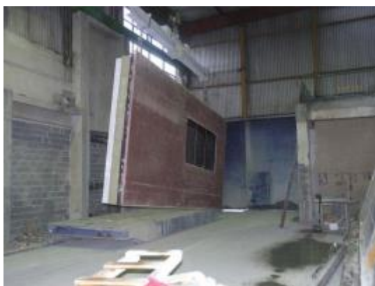
Slika 4-8: Prototip eco-sandwich ploče (ECO-SANDWICH, 2015)
