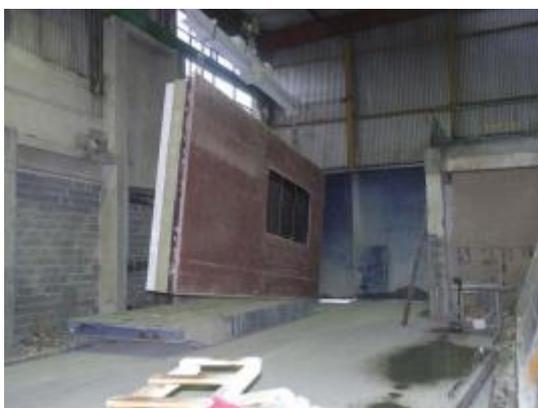
Slika 4-8: Prototip eco-sandwich ploče (ECO-SANDWICH, 2015)
