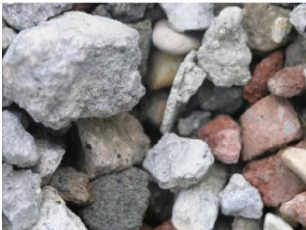
Slika 4-10: Reciklirani agregat (ECO-SANDWICH, 2015)
