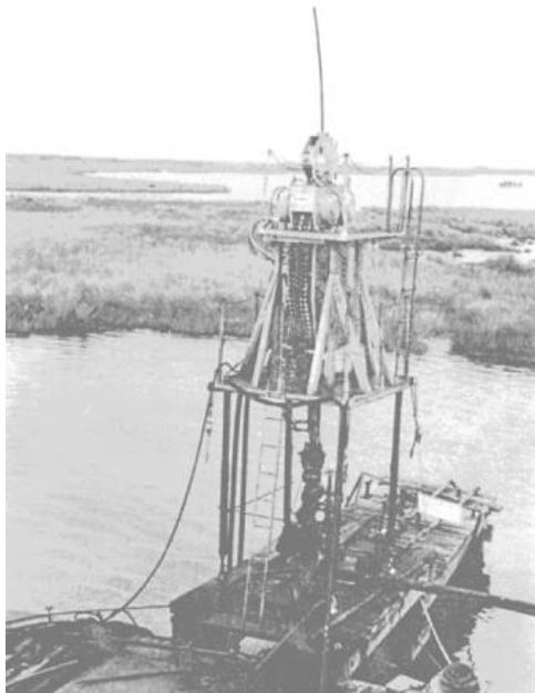
Slika 2-4. Prototip injektorskog sklopa kompanija California Oil Company i Bowen Tools (Coil Solutions, 2007)
