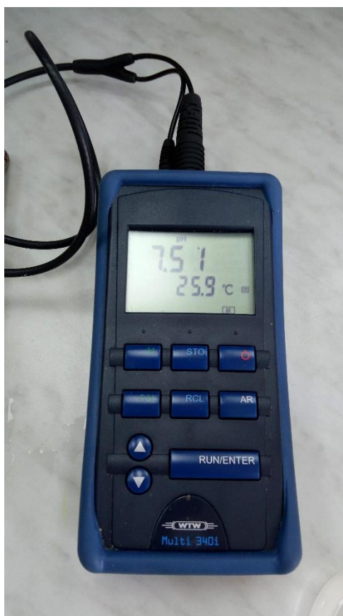
Slika 3.7. pH-metar WTW Multi 340i (foto: Borna-Ivan Balaž)
